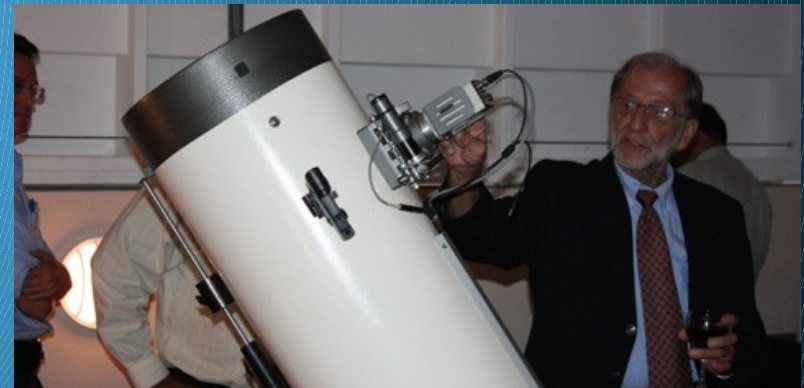
Bill's Newtonian Reflector with a H-alpha Detector at the focus
