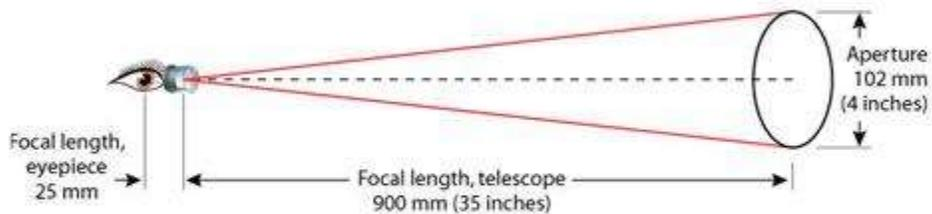
$$\text{Magnification} = \frac{\text{focal length, telescope (900)}}{\text{focal length, eyepiece (25)}} = 36 \times$$
